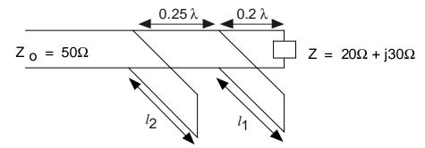
a) find the reactances that the stubs should add to the circuit in order to prevent reflection at the input end.
