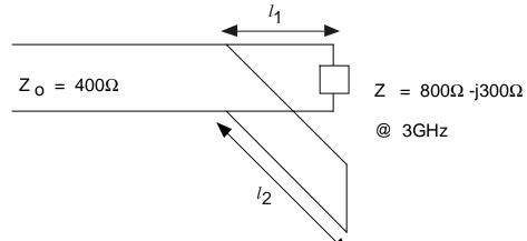
Find the position of the stub relative to the load  $l_1$ , and the length of the tuning stub  $l_2$ .
