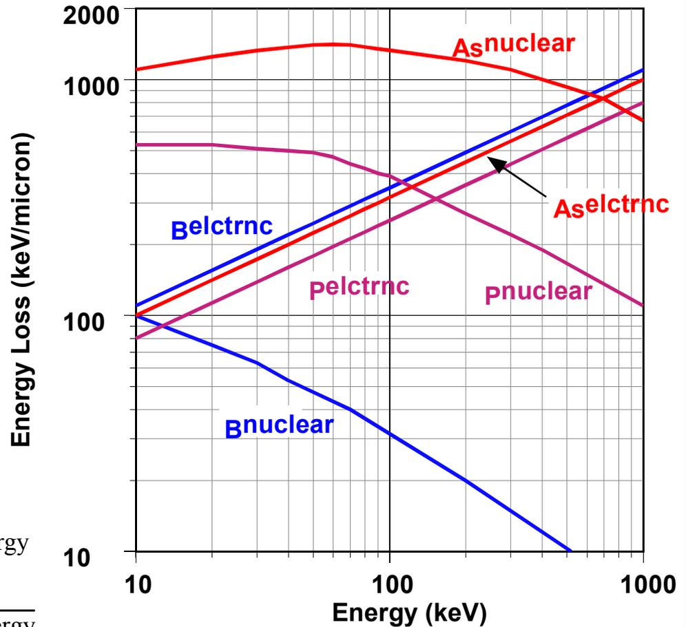
$$R = \int_0^E \frac{dE}{|dE/dx|} \approx \begin{cases} \text{nuclear: } \int_0^E \frac{dE}{\text{constant}} \propto \text{energy} \\ \text{electronic: } \int_0^E \frac{dE}{\sqrt{E}} \propto \sqrt{\text{energy}} \end{cases}$$
