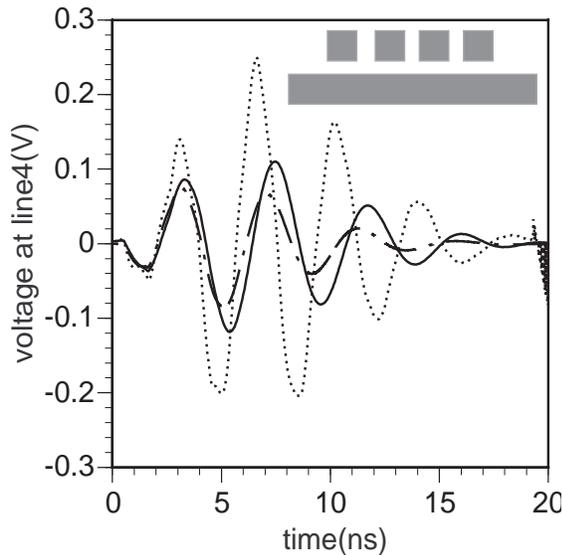
(c) far end voltage waveform at line 4: errors induced by failure to correctly include both resistance and inductance frequency dependencies: Solid line: FFT using full dispersion curve; dotted line: constant R-L-C transmission line analysis; dashed-dotted line: Star-Hspice<sup>®</sup> 97.2 using W Element where one high frequency resistance value must be calculated using some other method (here, the surface ribbon method was used [2]).
