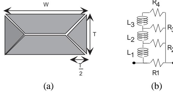
Figure 2) (a) Segmentation scheme for rectangular bar to approximate surface impedance. (b) Equivalent circuit model for approximated surface impedance.
