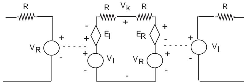
Figure 3) Equivalent model for method of characteristics.  $E_R$  and  $E_I$  are voltage dependent sources of reflected and incident waves respectively and appear in second part of right hand side of the equation 8a and 8b, respectively.
