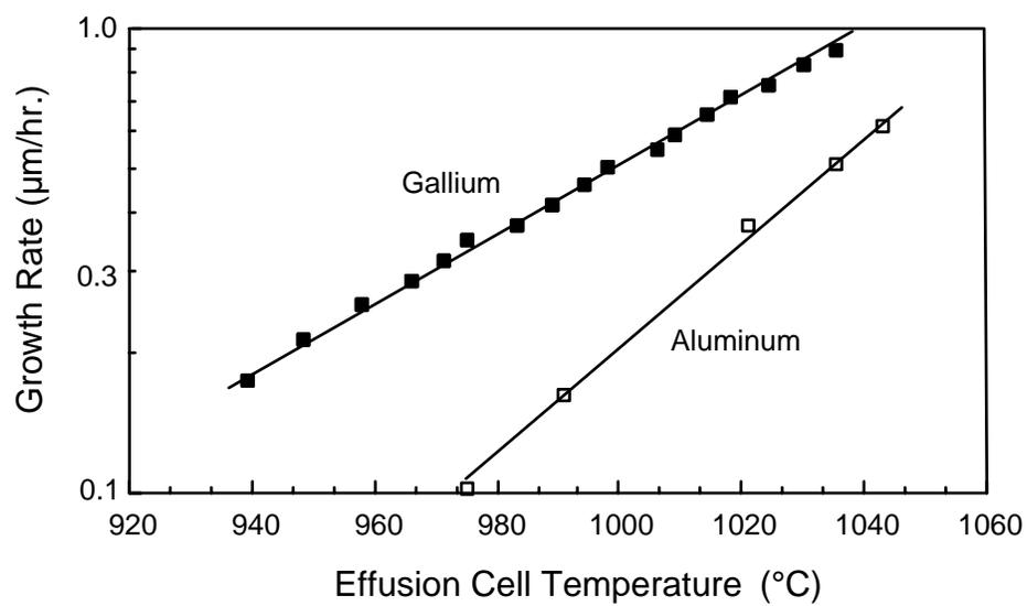
Fig. 3.1: RHEED measurements of the growth rate of GaAs and AlAs as a function of gallium and aluminum effusion cell temperatures.
