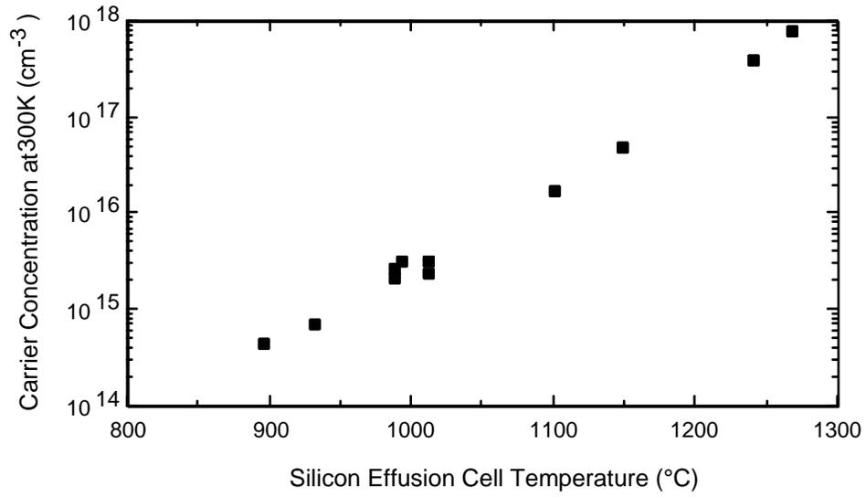
Fig. 3.2: Carrier concentration at 300K, as determined by Hall measurements, for MBE grown silicon doped GaAs layers versus silicon effusion cell temperature.
