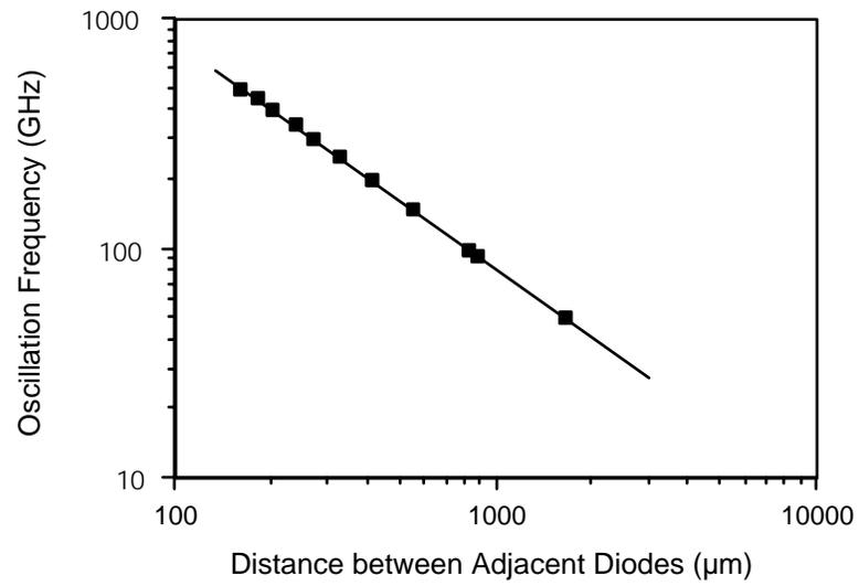
Fig. 6.3: Oscillation frequency as a function of the distance between adjacent diodes. At any desired oscillation frequency the distance between the diodes must be half the guide wavelength.
