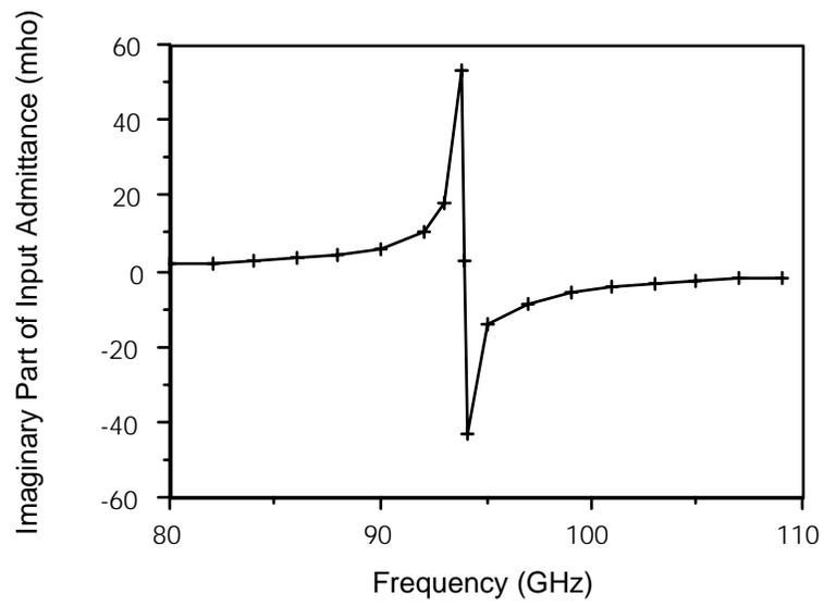
Fig. 6.2: Imaginary part of the input admittance as a function of frequency for a periodic oscillator circuit designed to operate at 94 GHz.
