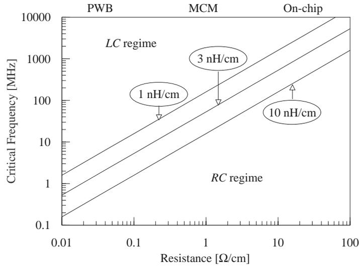
Figure 1.1: Critical frequency ( $\omega = R / L$ ) vs. resistance of interconnects with varying inductance of 1, 3, and 10 nH/cm.
